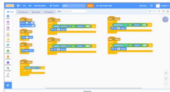
Figure 5: The "Breakout" project in the enhanced Scratch IDE. The addons for IDE space management allow for a larger coding area and thinner blocks.
